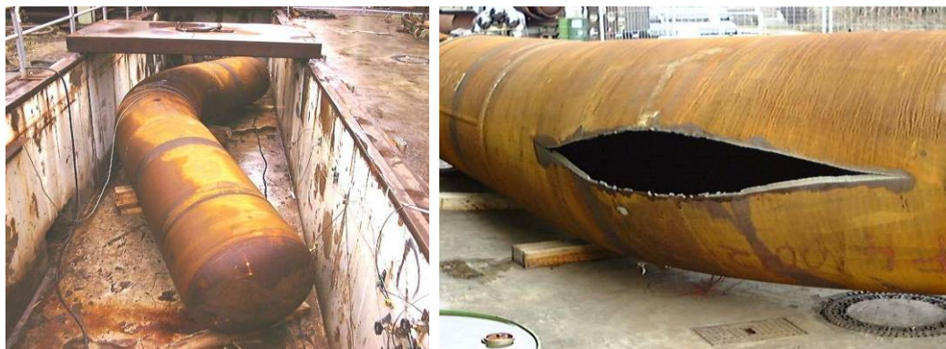
Figure 13 - Overview burst test (before and after testing) of X80 bend, measuring 48" with 28 mm min. wt. and 3D radius, performed at Salzgitter Mannesmann Forschung GmbH, Duisburg
