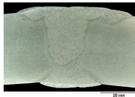
Fig. 12: Macrosection across the longitudinal multi-layer weld after full-body QT treatment (48" bend)
