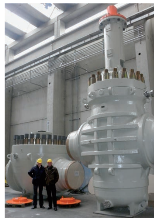
Fig. 4: The large 48" double expanding gate valves are installed in order to isolate the pig traps from the pipeline. They are 10.4 m high and have a weight of 102 tons (Petrovalves srl, Italy)
