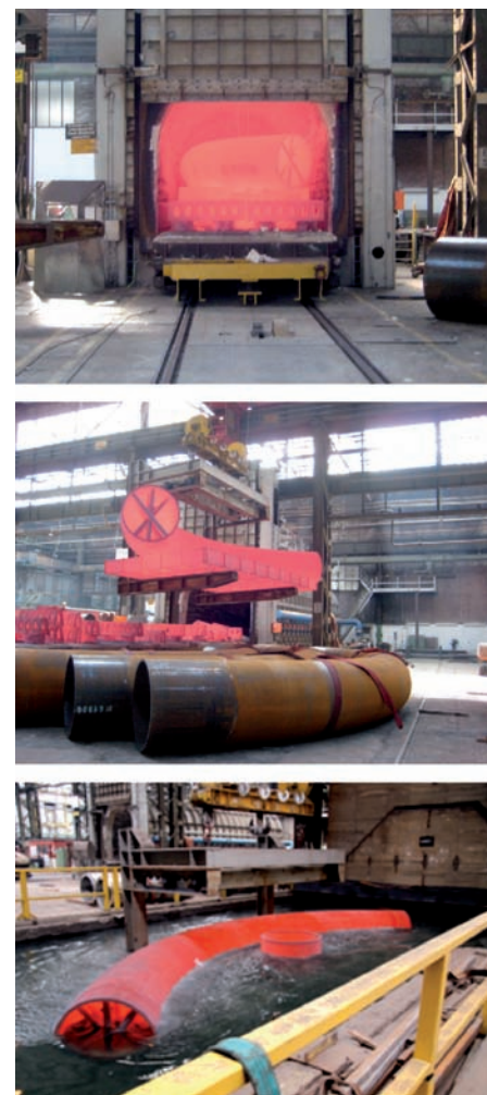
Fig. 5: Transfer of a 48" bend for the Nord Stream Project from the heat treatment furnace to the quenching bath at the MGB bending plant
